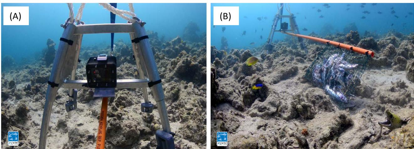
**Figure 1.** The baited remote underwater video stations (BRUVS) used in global survey to estimate shark and ray abundance on coral reefs (Global FinPrint Project). BRUV station comprises (A) of a GoPro Camera within an underwater housing on weighted metal frame, (b) with a bait pole attached to attract predators. Photo credit: Global FinPrint Project, [www.globalfinprint.org](http://www.globalfinprint.org).
